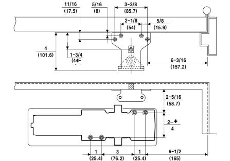
Hold-open arm. Identify direction of hold-open nut according to mounting.
