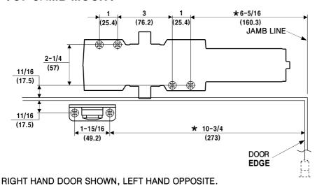
Hold-open arm. Identify direction of hold-open nut according to mounting.
